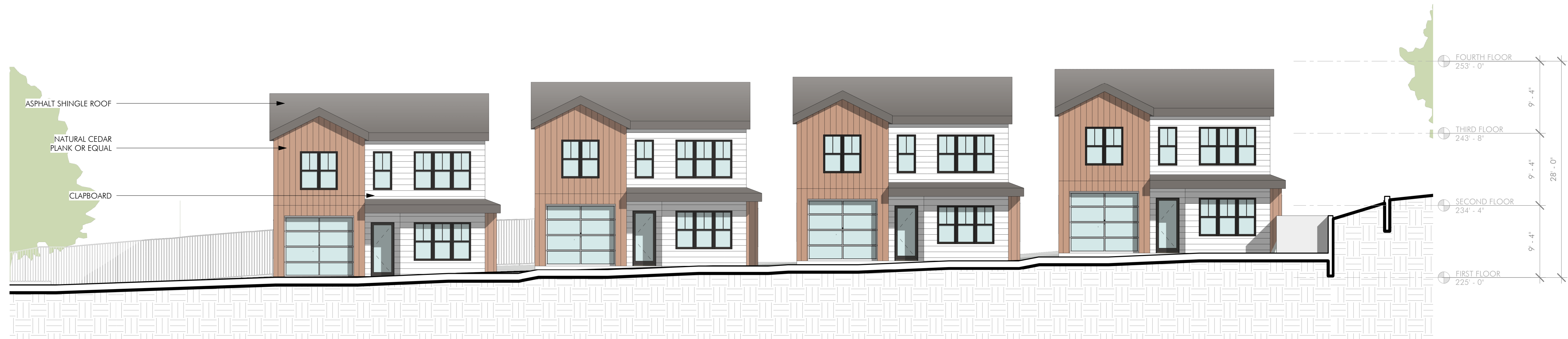
2 NORTH ELEVATION (TYPE B UNITS FRONT) 1/8" = 1'-0"
