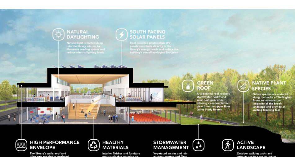
The library's walls, roof and windows are highly insulated to limit energy transfer and maximize the efficiency of heating and cooling systems
