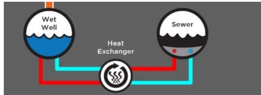
“WASTE” HEAT TO THERMAL COMFORT
