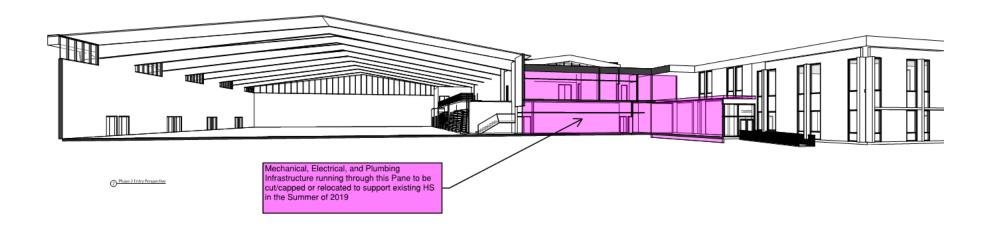
Mechanical, Electrical and Plumbing (MEP) infrastructure passing through the highlighted area to be cut/capped or relocated to support existing high school in the Summer of 2019
