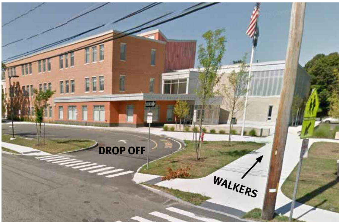
Clearly defined drop-off zones and walking routes improve pedestrian safety Credit: Google Maps Streetview
