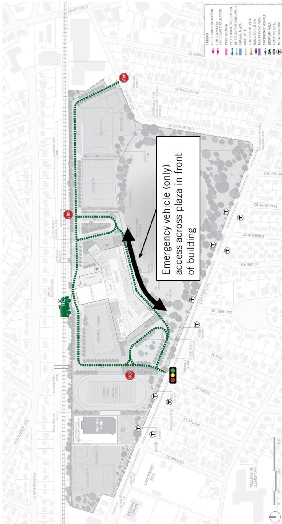
Figure 32 Measure 9: Enhanced Emergency Vehicle Circulation
