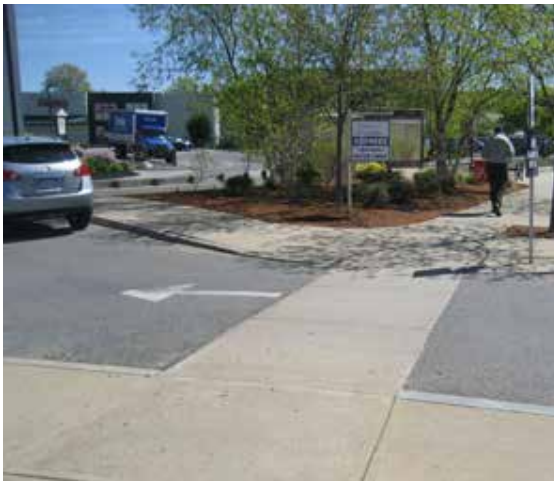
Continuous sidewalk across a driveway
