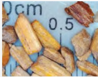
BrockFILL after 20,000 Lisport cycles.
