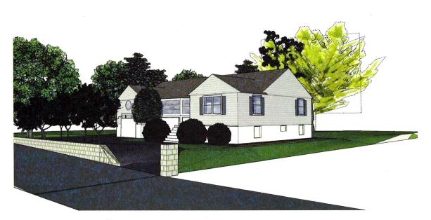
*Figure g Proposed Option 1:* Street View with two end basement windows enlarged by 1'5" inches vertically.
