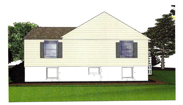
Figure h Proposed Option 1: Street View with two end windows enlarged by 1'5" inches vertically.
