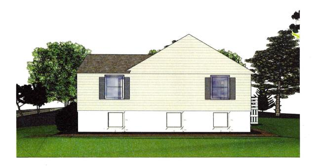
*Figure l Proposed Option 2:* Side view with three windows enlarged by 1'5" inches in height. Symmetry maintained. Since windows are still above grade, the ground level remains unperturbed.
