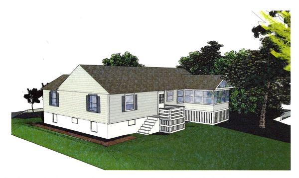
*Figure i Proposed Option 1*: Rear angle view with two end windows enlarged by 1'5" in height. Note that the current ground level remains unperturbed since the window sill is still above grade.
