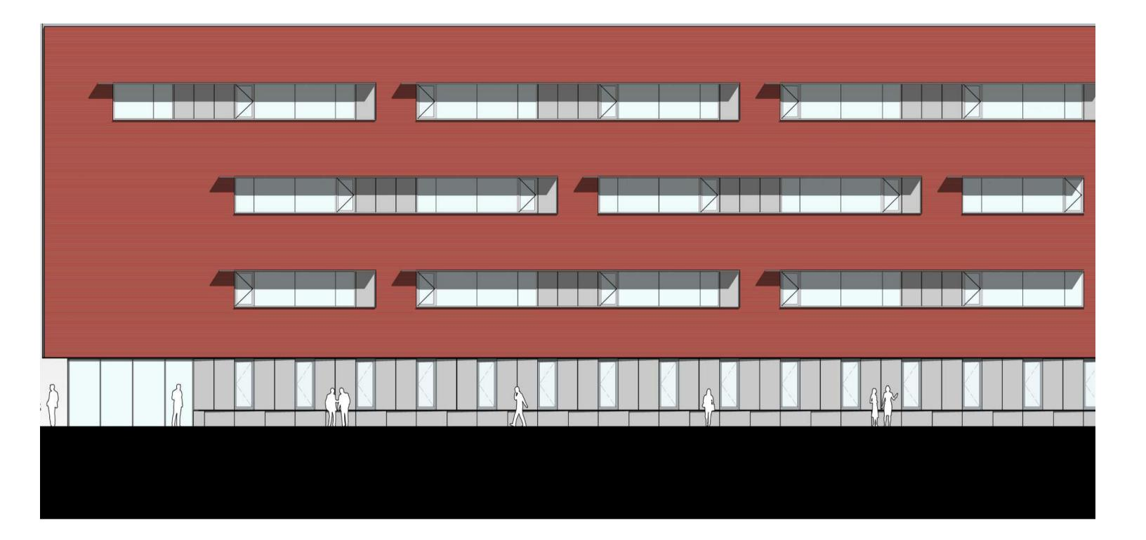
• CURRENT DESIGN REMOVES ~340 SF OF GLASS SPANDREL AND ~120 SF OF BRICK IN THIS SAMPLE ELEVATION - TO BE REPLACED WITH CEMENTITIOUS PANEL (~460 SF)
