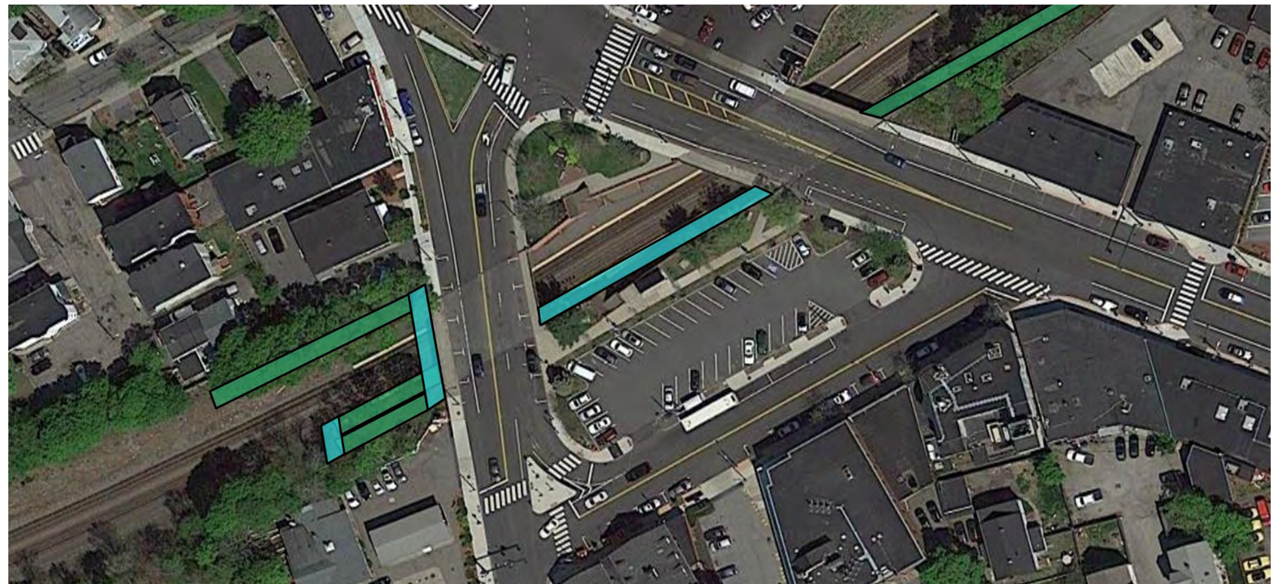
Alignment of path from Waltham connection to being elevated over inbound platform (W7a) — green: grade change, blue: level.
