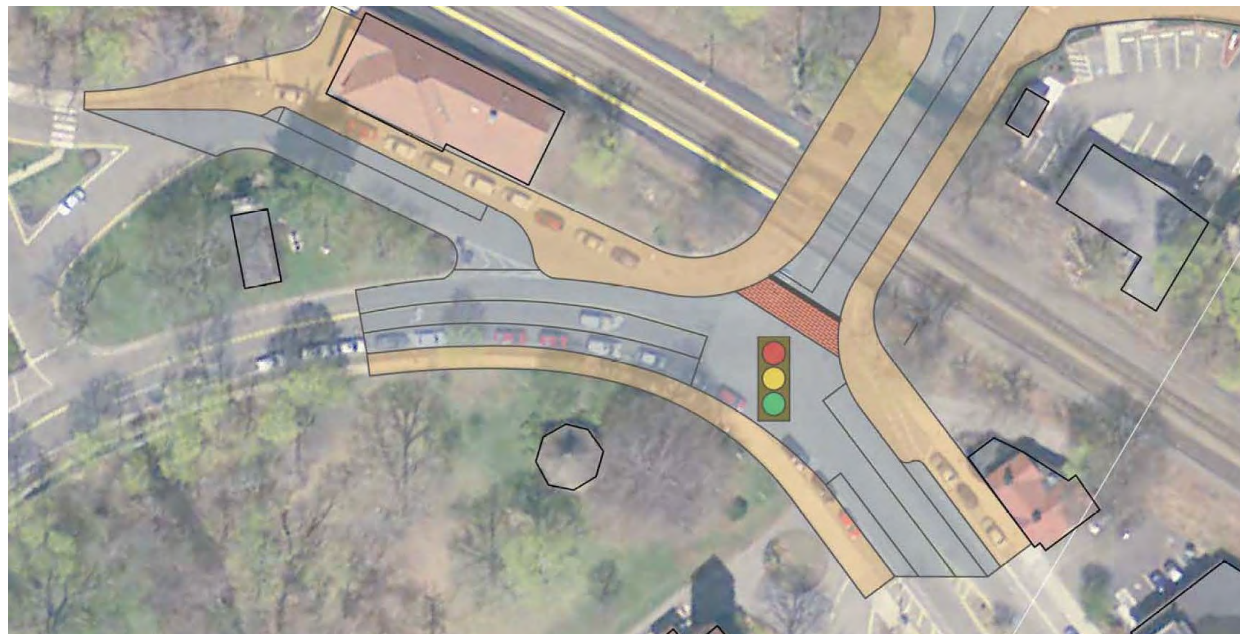
Switch Sides (C4b) or Continue South (C4c): Narrow pavement width on Concord Avenue in underpass and/or signalize crossing.
