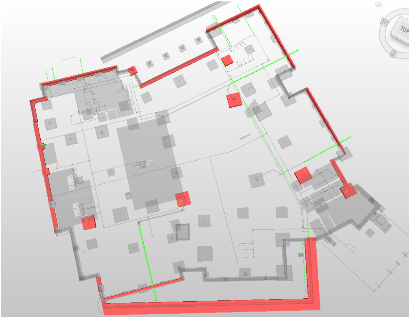
Overview - there are a few spots where piping needs to coordinate w/ foundations.
