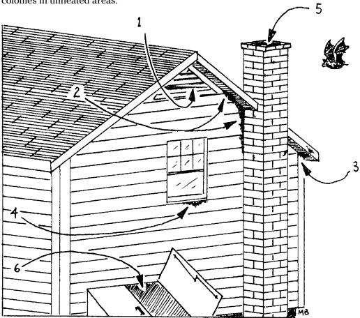
The most common entrance ways for bats entering a home include (1) an unscreened attic vent, (2) a crack or separation where the chimney meets the house, (3) a hole or crack under a rotted eave, (4) rotted window sills or loose-fitting screens, (5) chimney flues, (6) an open cellar hatch (bulkhead). Other possible entrances include openings where pipes or wiring meet the house, and gaps in loose or warped siding.
