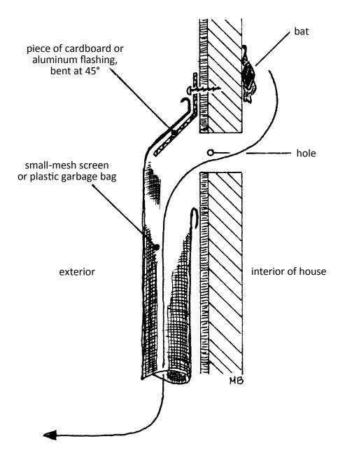
This highly effective, one-way bat excluder can be constructed with nothing more than a sheet of cardboard, a plastic garbage bag and a couple of screws or nails. This simple design is best for small entrances, but can be adapted to function on even large cracks or openings.
