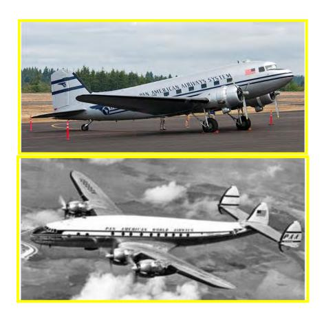
Figure 2.3-5. Twin-engine propeller-driven Douglas DC-3 and four-engine propeller-driven Lockheed Constellation
