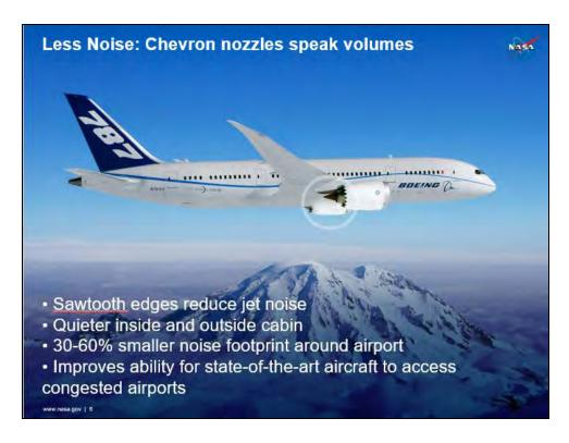
Figure 3.3-4 NASA-Supported Advance: Chevron Nozzles
