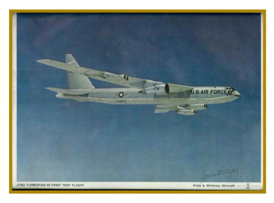
Figure 2.3-7 JT9D engine slung under the wing of a B-52 in its first flight test out of Bradley Field in June 1968
