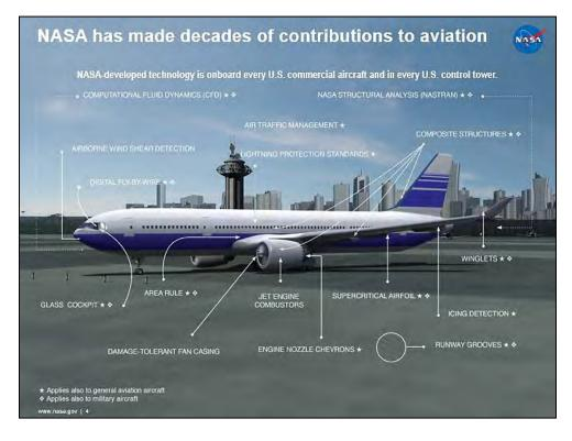
Figure 3.3-3 Examples of NASA's Continuing Contributions to Aviation Technology
