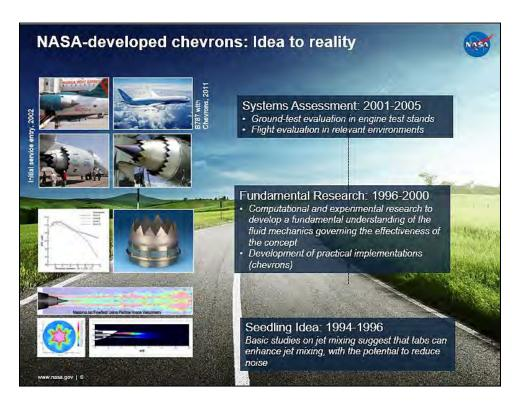
Figure 3.3-5 How NASA Developed Chevron Nozzles
