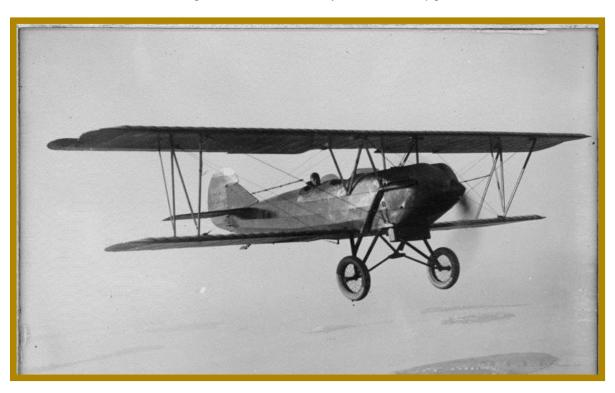
**Figure 2.3-4** Travel Air open cockpit biplane with OX-5 engine that was owned and operated by the Harvard Flying Club out of East Boston Airport
