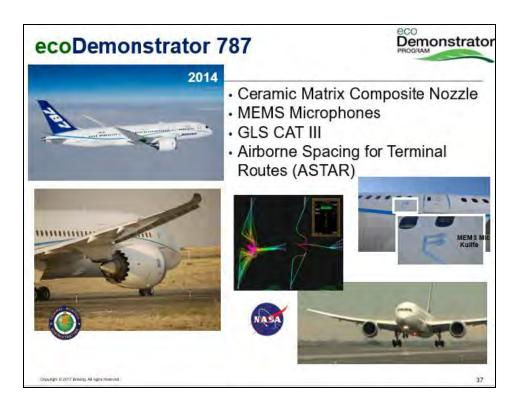
Figure 3.8-6 Advances Have Emerged from ecoDemonstrator 787
