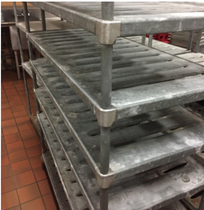
Storage shelving made using galvalum is not resistant to chemicals and eventually corrodes as shown here. New shelving offers corrosion proof materials with easily removable sections that can be placed in a sink or dish washing machine for easy cleaning and sanitation must be exhausted from the room.
