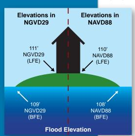
elevation (LFE) from an Elevation Certificate based on NAVD88. The error could be significant if they are not first converted to the same vertical datum. Similarly, when calculating a new premium with a BFE based on NAVD88 and a building's LFE based on NGVD29 from an older Elevation Certificate, the elevations should be converted to the same vertical datum.
