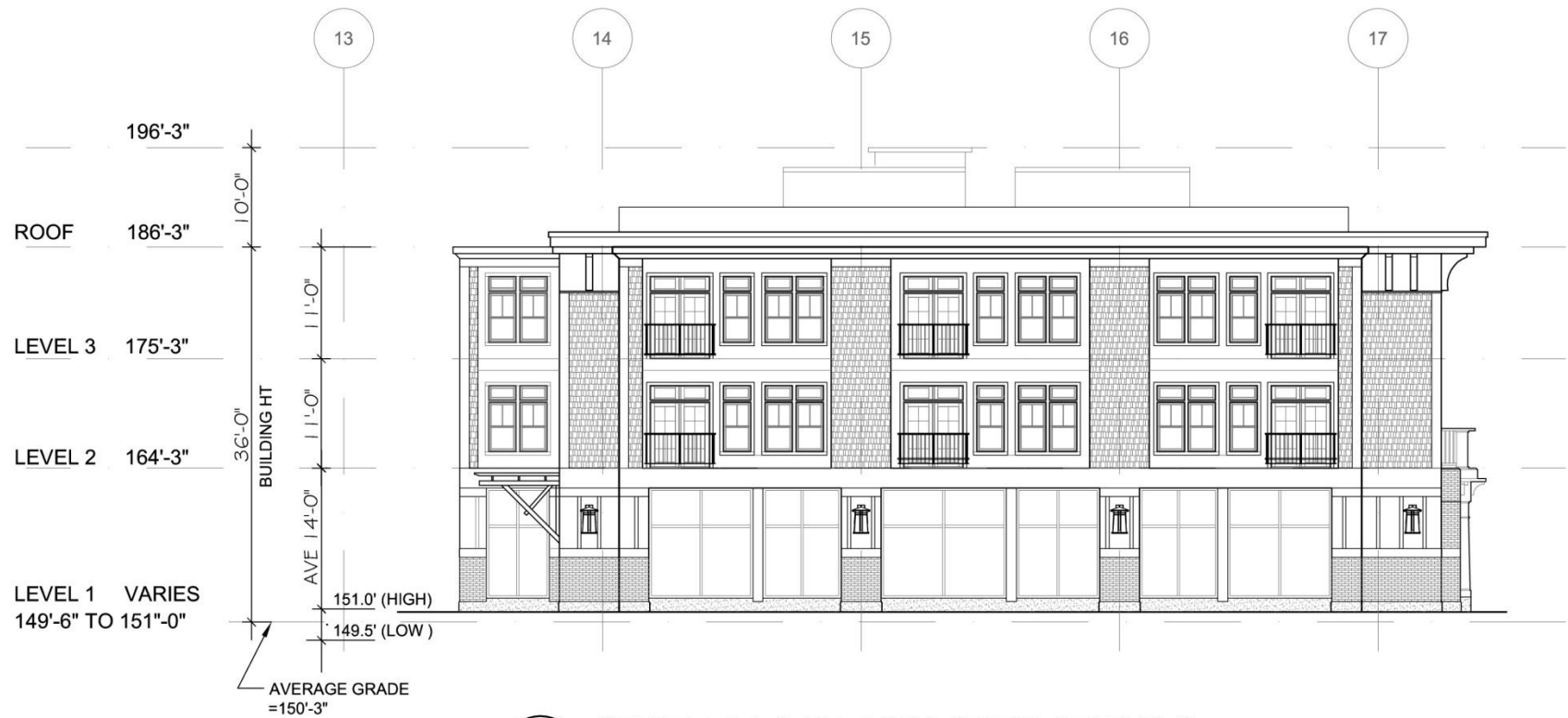
4 SIDE ELEVATION (DRIVEWAY) SCALE 1/16"=1'-0"
