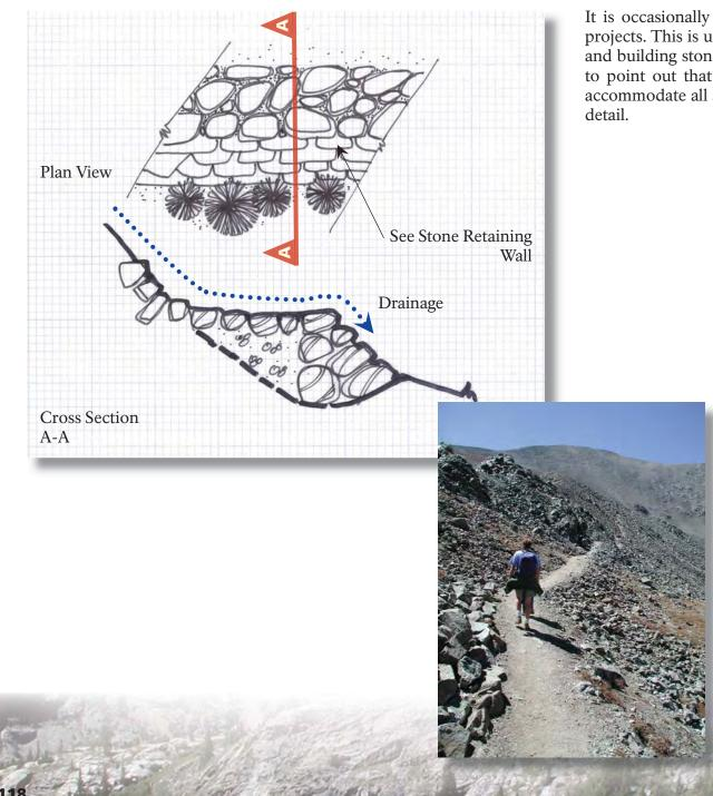
It is occasionally necessary to cross talus in complex mountain trail projects. This is usually done by rearranging rocks in the trail corridor, and building stone retaining wall supports if necessary. It is important to point out that a talus crossing must be sufficiently wide to safely accommodate all allowable types of traffic. See the stone retaining wall detail.
