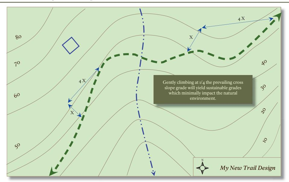
Using a pair of engineering dividers or a map tool from topographic map software, the interdisciplinary trail team can layout trail alignments on the base map by first measuring the prevailing cross slope (X) and extending out four times (4 X) parallel to the contour.
