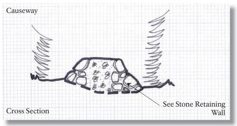
Causeways are options to consider when crossing unstable soils or for use in riparian areas. Two stone retaining walls are built to elevate the trail surface above the unstable condition. Some pointers:
