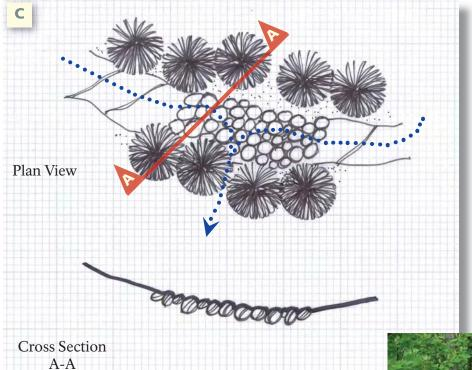
Stone paving or a paved dip can be used to improve unsuitable soil conditions or in low points along the trail corridor that experience wet conditions or areas that otherwise would not support a sustainable trail surface. Some pointers:
