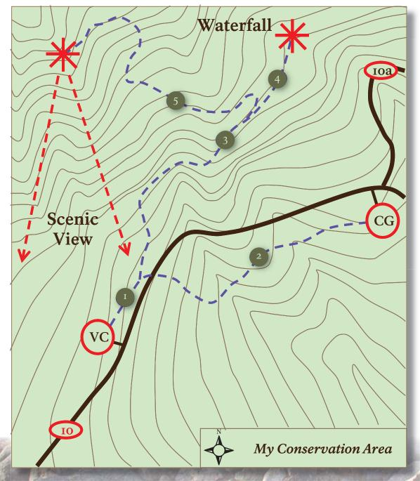
In this example area, trails developed over a period of time without the benefit of professional planning or design services. No guidelines were applied. Trails have been heavily used, and the season of use has increased substantially from summer use to shoulder season through summer through shoulder season with some intermittent winter use. Some of the trail segments go straight uphill.
