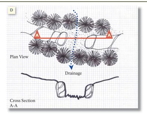
Stepping stones can be used to provide alternative pedestrian routes across wet areas or intermittent streams. Some pointers:
