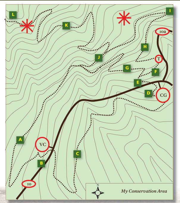
Trails that link appropriate origins and destinations with appropriate intermediary linkages form the basis of a mountain trail plan. Most of the identified corridor control points are accommodated in this plan.
