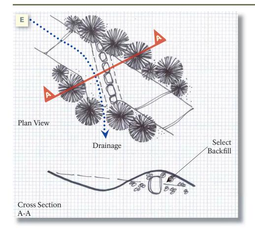
Good waterbars will cut down erosion and subsequent maintenance of otherwise well built trails. Some pointers:
