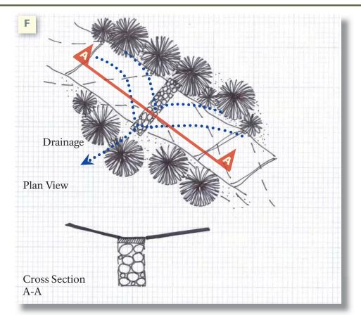
Stone drains collect runoff and carry it across the trail. French drains carry runoff under the trail, and sometimes parallel to the trail (yet still underground) and then under the trail. Some pointers:
