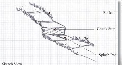
Check steps are an option when severe erosion has gullied out a trail and relocation of the trail is not an option.
