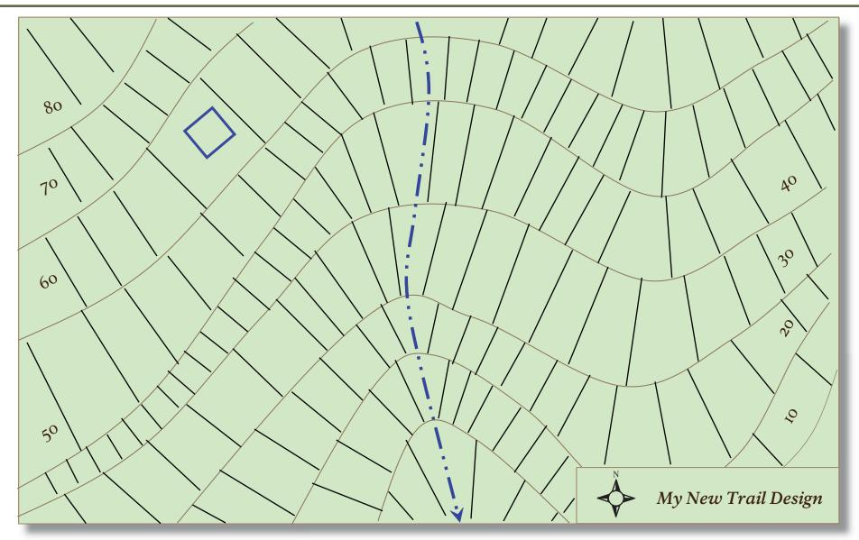
Slope analysis is the most fundamental landscape architectural site planning tool and will yield insights into the degree of modification required to fit a trail corridor to the ground. Steeper prevailing cross slopes require more investment of time and materials. Sometimes extensive armor improvements are required.
