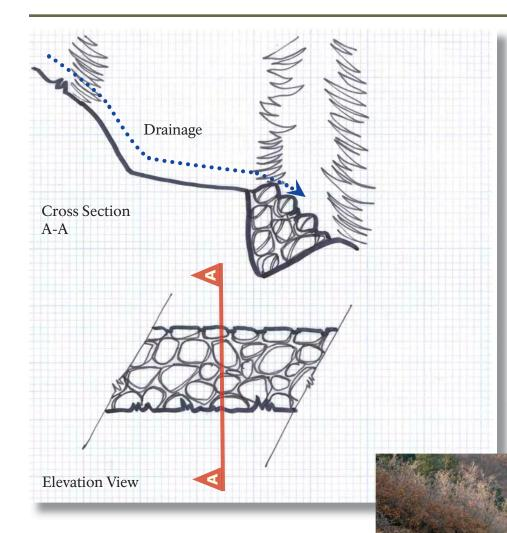
Stone retaining walls allow trails to be built where they normally would not be able to be built, or to improve unsustainable conditions. Some pointers:
