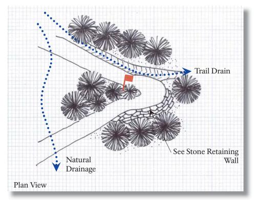
Switchbacks are utilized where it is necessary to change the direction of the trail. Some pointers:
