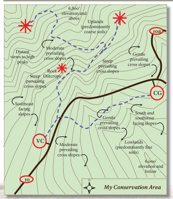
Existing cross slope ranges are generally moderate. Approximately 55% of the property has cross slopes of 20 – 60%; approximately 15% over 60%; and approximately 40% of the parcel is in the less than 20% range.
