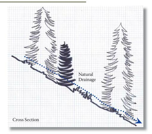
Many mountain trail projects are on moderate to steep prevailing cross slope ranges. This example is drawn on a 40% cross slope. Earthwork quantities can be estimated from the cross slope condition. A variety of vegetation types are typically encountered, and sometimes significant clearing of trees is required before tread construction can begin.
