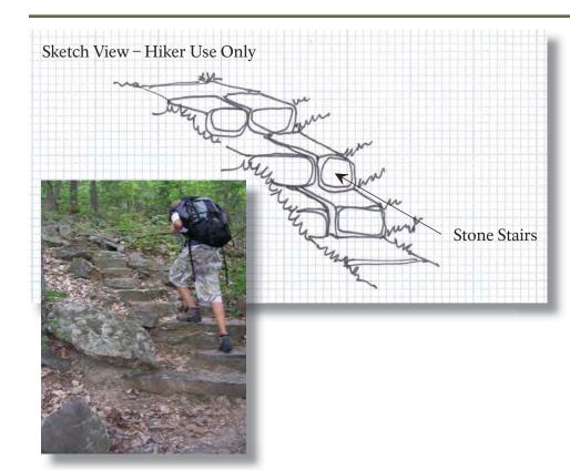
Stone stairs can be used where grade must be gained quickly. Stairs are not intended to be used on trails that have horse or mountain bicycle use. Build stone stairs to withstand significant use and impact. Some pointers:
