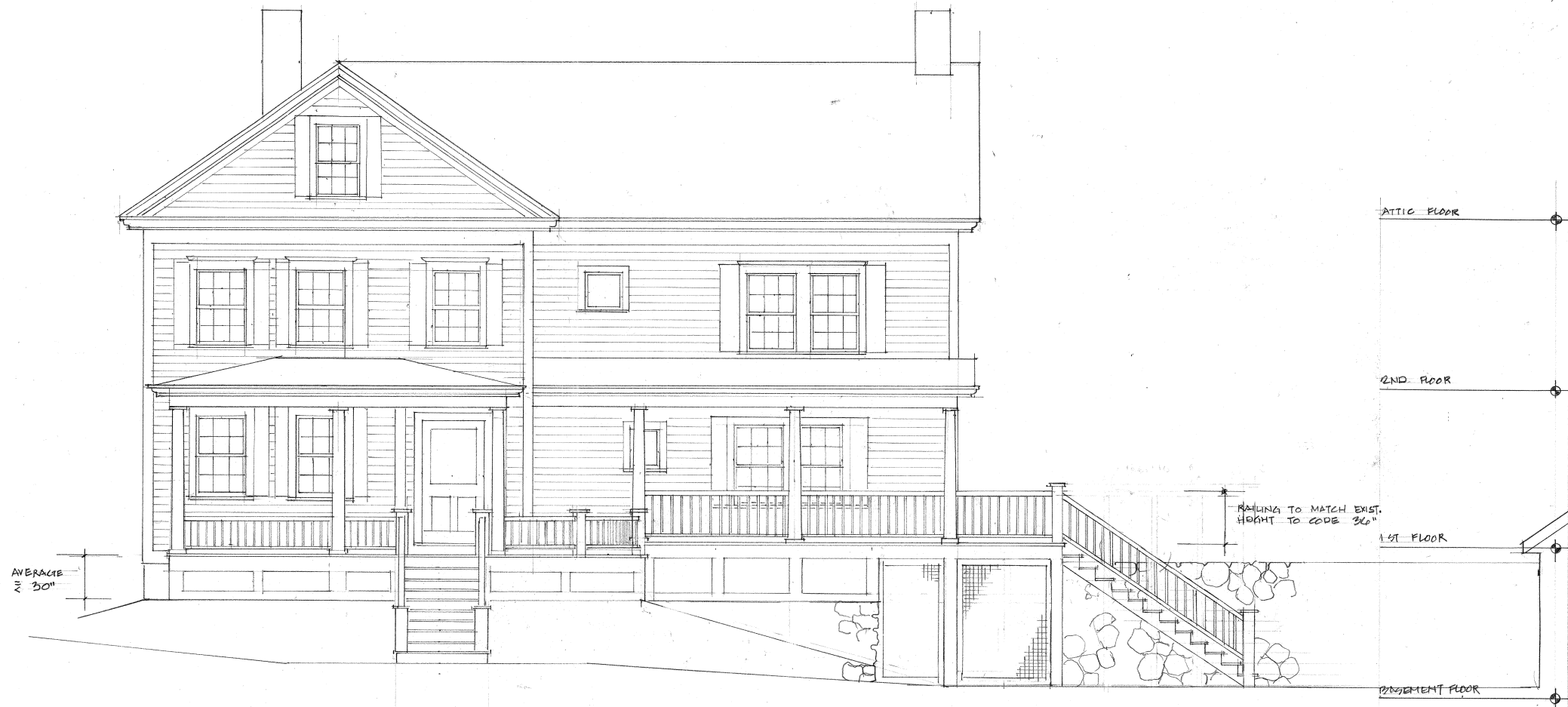
EAST ELEVATION PROPOSED SCALE 1/4" = 1'-0"
