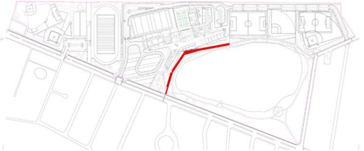
Concrete Vehicular Paving: medium broom finish 6" depth w/ reinforced welded wire mesh, 12" compacted gravel borrow, type B.
