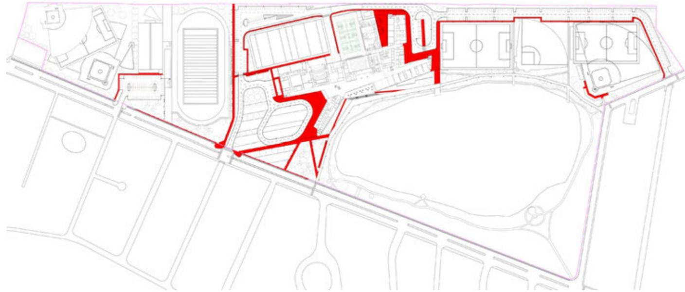
Concrete Pedestrian Paving: medium broom finish 4" depth w/ reinforced welded wire mesh 8" compacted gravel borrow. Sawn expansion joints maximum 30' O.C., control joints maximum 10' O.C. Integrally colored concrete admixture shall be incorporated in the concrete mix where indicated with sandblasted feature bands.
