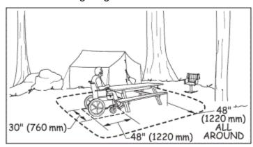
Recommend providing clear floor space of 36" wide minimum by 48" deep alongside one bench so that a wheelchair user can sit alongside someone sitting on the bench. See the following diagram:
