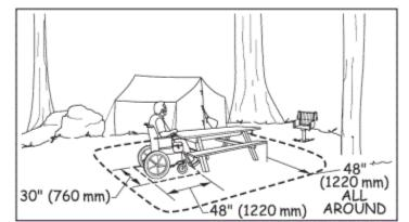
Recommend providing clear floor space of 36" wide minimum by 48" deep alongside one bench so that a wheelchair user can sit alongside someone sitting on the bench. See the following diagram:
