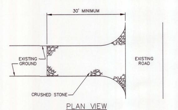
THE ENTRANCE SHALL BE MAINTAINED IN A CONDITION WHICH WILL PREVENT TRACKING OR FLOWING OF SEDIMENT ONTO EXISTING ROAD. THIS MAY REQUIRE PERIODIC TOP DRESSING WITH ADDITIONAL STONE OR ADDITIONAL LENGTH AS CONDITIONS DEMAND AND REPAIR AND/OR CLEANOUT OF ANY MEASURES USED TO TRAP SEDIMENT. ALL SEDIMENT SPILLED, DROPPED, WASHED OR TRACKED ONTO EXISTING ROAD SHALL BE REMOVED IMMEDIATELY.
